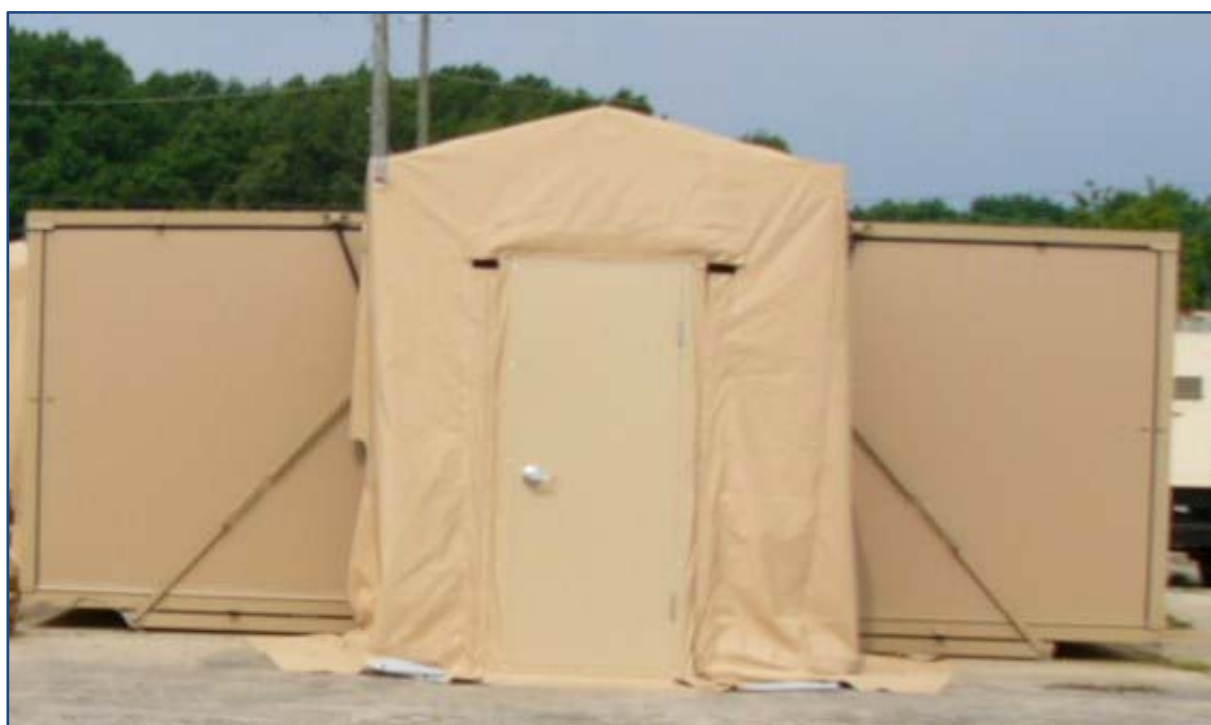
Vestibule shown with solid door and colour Desert Tan, attached to expanding shelter (Mobile Forensic Laboratory)
